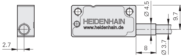
Right-side cable outlet, angled (0°)
